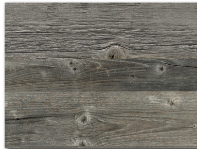
Spruce 5C (raw, untreated) 1,3 Sunburnt, lightly brushed and patched with real wood. Structure vertical or horizontal
