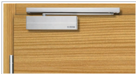
OTS1 Door closer with slide rail and mechanical hold open Colour F1 (aluminum silver) (can only be ordered up to a door leaf width of 1100 mm)
