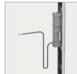
LOCK SWITCH CONTACT RSK2 Built into the upper striking plate. Used by the upper hook Feedback: door is locked!
